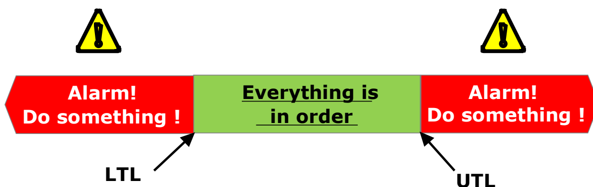
Fig. 19.1-1 General form of a numerically defined target
